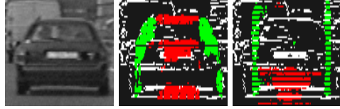
Fig. 4. Hausdorff distance classifier: each region is compared with two models
