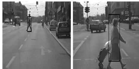
Fig. 3. Tracking of pedestrians based on the cross entropy based on intensity distributions and LOC features
