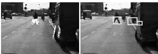
Fig. 3. Detection of pedestrians (model matching).
