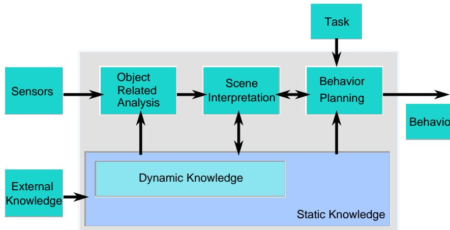
Figure 1: Architecture for a driver assistance system.
