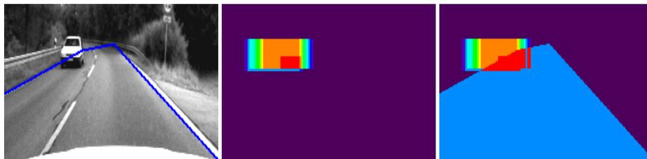
Figure 5: Oncoming traffic (image with lane-information, movement-sensitive representation without and with preactivation). The preactivated region is determined by the lane information. The value indicates the grade of activation.
