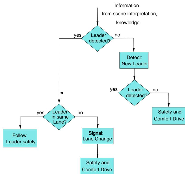
Figure 8: Flow diagram of signal behavior for ICC.
