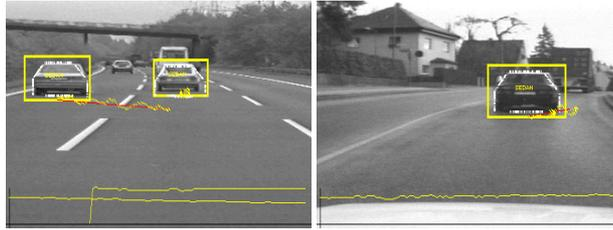
Figure 3: Vision-based object detection, object classification and object tracking.
