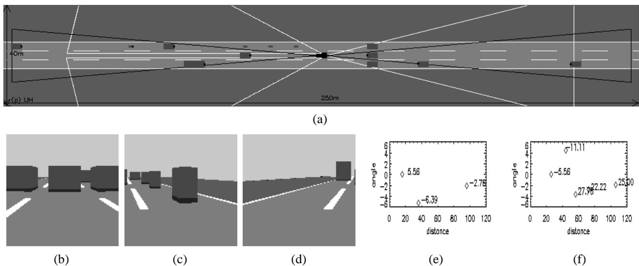
Figure 9: Sensor simulation: (a) bird's-eye view with mounted sensors on the vehicle; (b)-(d) camera output of the three cameras; (e)-(f) plotted results of the radar sensor output.
