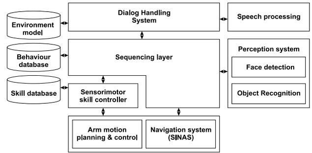
Figure 2: The robot control system.
