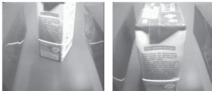
**Fig. 7.** The view from the gripper camera at the beginning and endpoint of the grasping motion.
