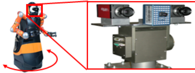
Fig. 1 Mobile technology platform with pan tilt unit and two mounted cameras (red).
