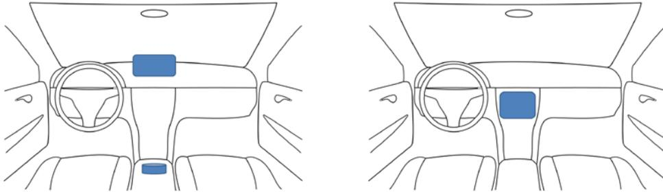
Figure 1: Typical cockpit styles: left: highly mounted display with controller, right: touchscreen
