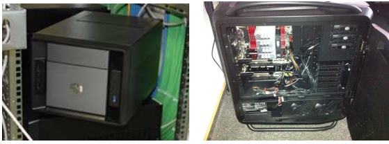
Figure 8. The two node types used in IGOR. The left picture shows very compact mini-ITX case with one discrete GPU, 16GB RAM and one HDD of 1TB. The right side depicts a large ATX tower with 64GB RAM, multiple GPUs and HDDs (8TB).
