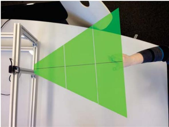
Fig. 4. Setup for the recording with the Camboard nano. The three zones of the recording: Near, intermediate and far.
