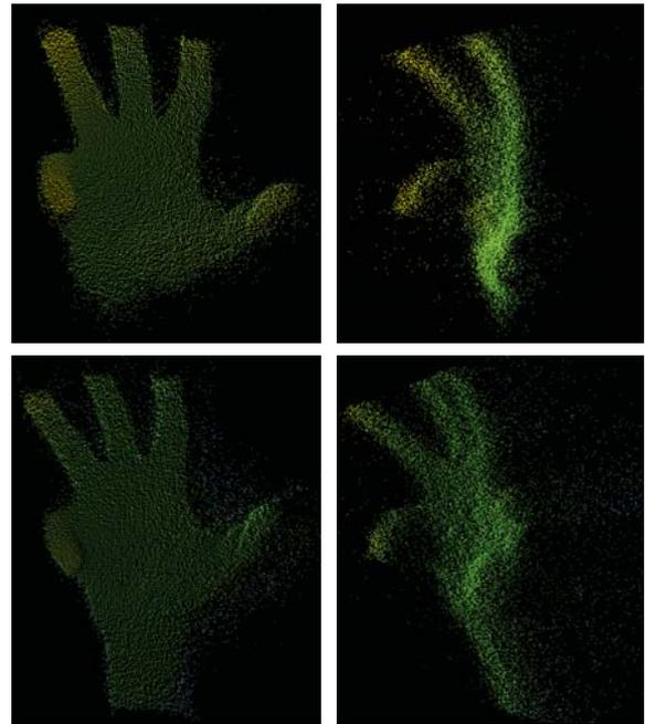
Fig. 5. Sample recording of a hand posture. Top row: The same posture from the front view (left) and the side view (right). Bottom row: The same hand posture in a subsequent state taken after the snapshot in the top row (same angles). Noise and outliers resulting from errors in measurement are clearly visible when seen from the side view (right column).
