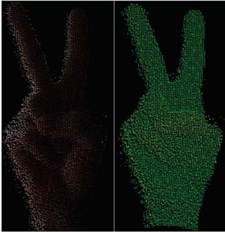
Fig. 3. Depth recording of hand posture *TWO* (right) and with the RGB information mapped onto the depth pixels (left).
