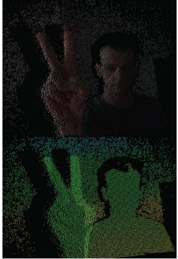
Fig. 2. Full scene recording - RGB and depth info merged (top) and depth info only (color coded, bottom): Depth thresholding allows for rapid segmentation of the hand-arm region from the background. Cropping irrelevant arm parts is achieved via PCA-segmentation.
