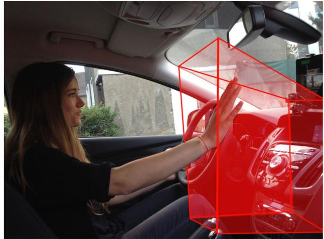
Fig. 2. A typical application scenario: The driver interacts with the infotainment system. The ToF-sensor captures the sensitive VOI marked in red.
