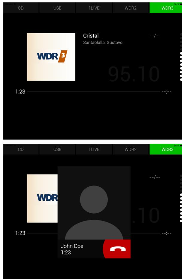
Fig. 1. Infotainment system: Multi-channel interface (top) and the same interface during an incoming call (bottom) (cf. Fig.3 for notations)
